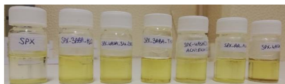
Figure 10 Solubility behaviour of SPX, SPX:3ABA Form I, SPX:4ASA Form II, SPX:3ABA Form II, SPX:4ASA Form III, SPX:AA and SPX:4ASA Form I (from left to right)
